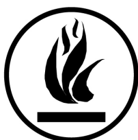
Flammable and Combustible Material
